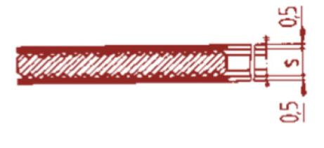
In order to avoid damage to the flanges with the metal core of grooved gaskets, they are generally used with layers of graphite, PTFE, aluminium or silver, providing total protection to the flanges and a secure seal even at low minimum surface pressures.
