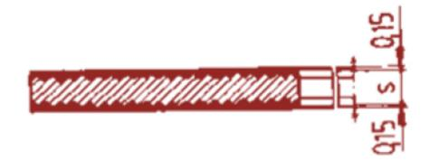
A triaxial stress is created in the profiling of the metallic carrier which has been filled with the layer material. The stability of this combination is therefore significantly higher than with a pure PTFE, graphite, or aluminium seal.
